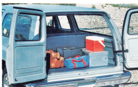
Panel-type rear doors have fixed, tinted glass; opening is 37" high by 59.6" wide. Power door lock available.
